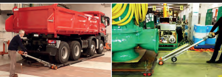
PowerAttack moves 18t Dumper on Transport Platform
